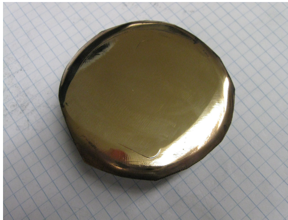
Figure 9: Mirror After Final Polish
